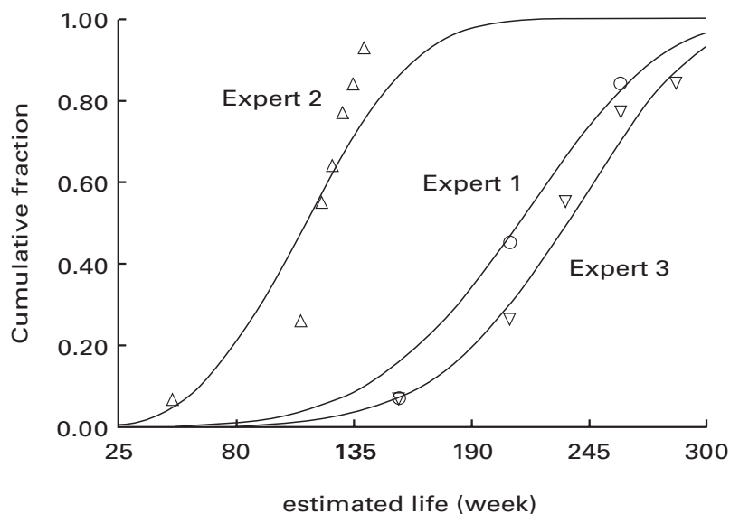
Figure 6.4: Cumulative frequency plots of life estimates and corresponding Weibull-2 fit; Median ranking is used on the data as obtained from plots as given in figure 6.3.
